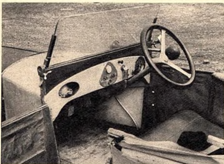
SLIM LINES are evident in the upper photograph, which shows the 1922 G.N. accompanied by its owner, B. H. Davenport. Right-hand brake and gear levers will be noted in the view of the cockpit, and also the conveniently positioned ammeter, oil-flow indicator, speedometer and horn bulb.
