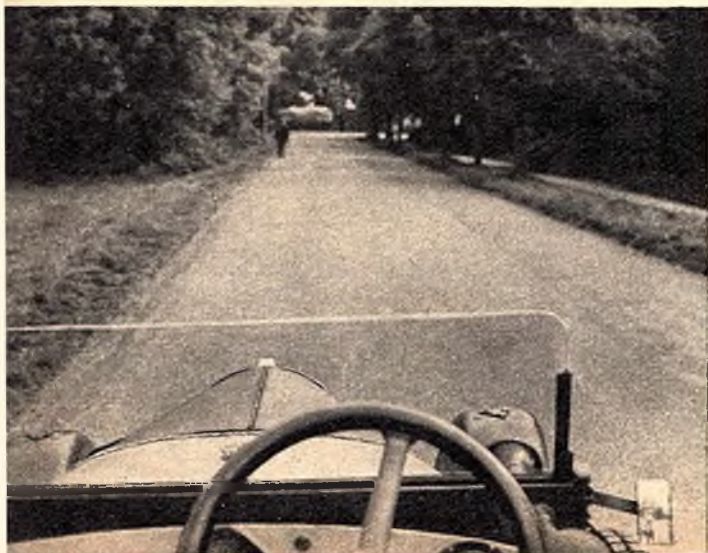
VISIBILITY without obstruction from bonnet or windscreen is a feature which endeared the G.N. to keen drivers.
