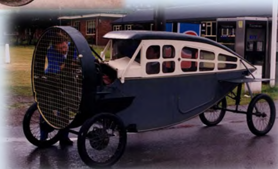
1920 Leyat owned by Roger Smith. Roger has been rebuilding this amazing device over a period of ten years from parts mainly found in France. It has original ABC engine, top speed 50mph if you are brave enough! Constructed like an aeroplane with wire and bobbin steering to rear wheels and handles well. Starting is by drum from the rear of the engine with a wire cable. As the engine is 1500cc and 9:1 compression ratio this can be demanding. There is another like this in France. Roger is trying to organise a re-creation of the film in the 1920's of two Leyats in the Champs Elyees.
