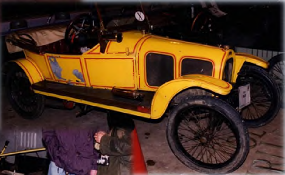
1913 GN Grand Prix owned by Tony Mitchell. Possibly the sole surviving 1914 Grand Prix GN and one of the first 150 made. V twin engine across frame with three speed gearbox, no reverse, double belt final drive. Originally destined for Russian order but war stopped that. Sold to Tom Faulker. Continuous history from new. Later Davis, Nigel Moores, Colin Crabbe, Roger Hancox and Roger Gates. Tony has owned the car since 1968 and campaigned it actively. A real cyclecar in ever way. GN's are so evocative of the cyclecar movement.
