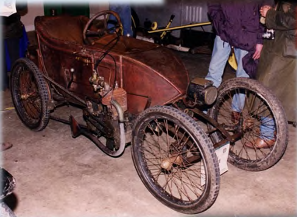
1920 Leyat owned by Roger Smith. Roger has been rebuilding this amazing device over a period of ten years from parts mainly found in France. It has original ABC engine, top speed 50mph if you are brave enough! Constructed like an aeroplane with wire and bobbin steering to rear wheels and handles well. Starting is by drum from the rear of the engine with a wire cable. As the engine is 1500cc and 9:1 compression ratio this can be demanding. There is another like this in France. Roger is trying to organise a re-creation of the film in the 1920's of two Leyats in the Champs Elyees.
