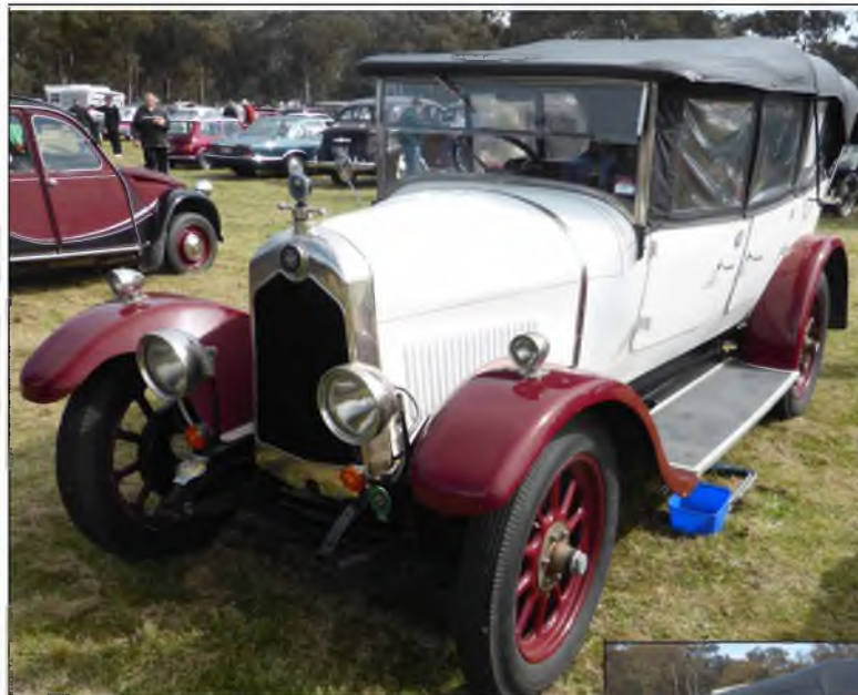
1925 Crossley 15/30 Tourer 4 cyl. 2383cc. 80 x 120mm. RAC horse-power 15.6. compression ratio 4.67. 31bhp @ 2400 rpm. 28mpg. 3 speed gearbox. max speed 55mph and weighs 21cwt.
