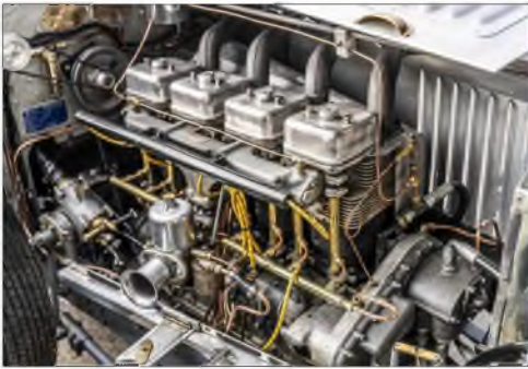
Cirrus aero engine in Joe and Bev Wilson's 1926 Vauxhall 14/40 special
