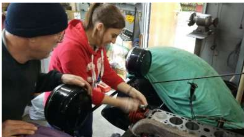
Below: Putting the water pump back on.
